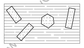
Q.43 The figure given below is the geological map of a flat terrain. It shows three unconformities and four magmatic bodies, one of which has intruded along a fault.
